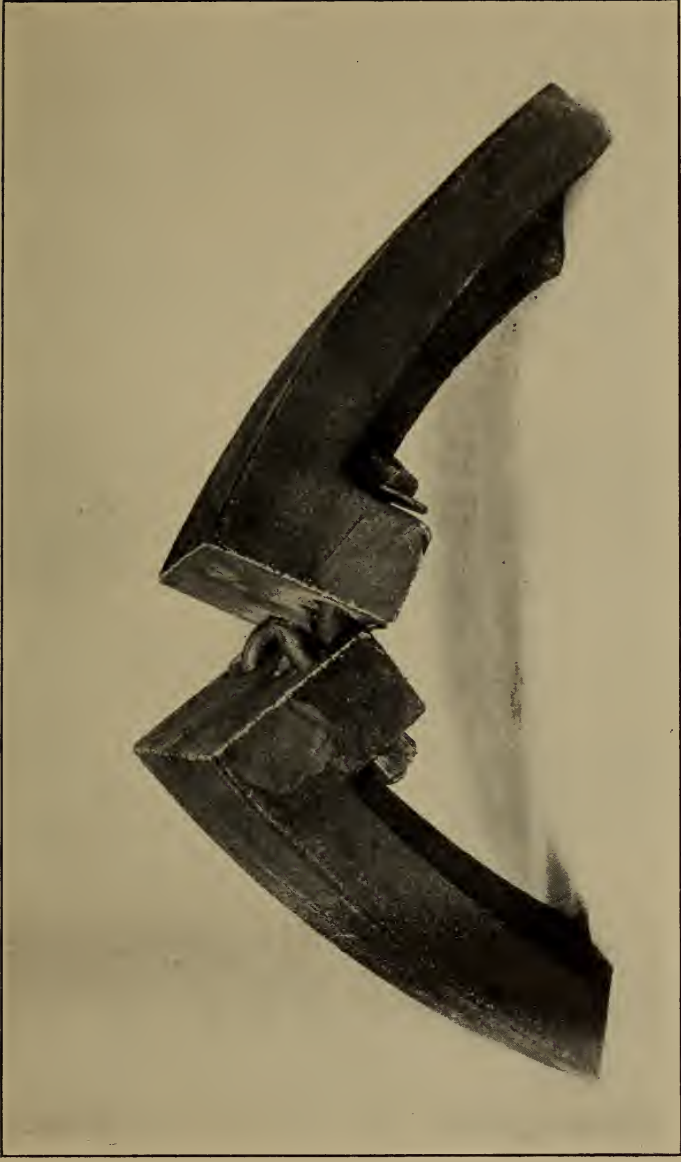
FIG. 79.—OPENING OF RIM JOINT AT HIGH SPEED.
